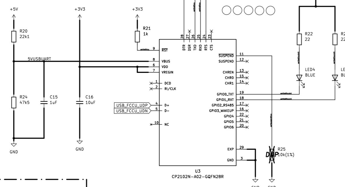
GPIO\_TXT and GPIO\_RXT are LED status indicators for data transmission. They are connected according to the technical documentation of the CP2102N-A2-xxx28R. See page 23 of the technical documentation.
